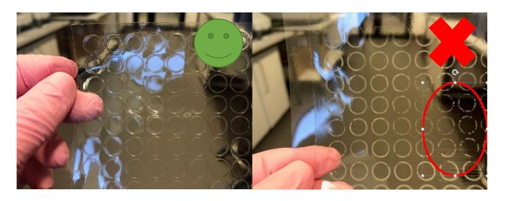
Good foil seal: No gaps in seal around wells.
