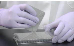
If you do not have a plate applicator you can rub across the surface of the plate horizontally and vertically using the backing from the adhesive film. Make sure that you do this over all the wells on the plate.
